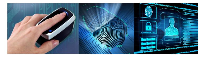
To clock, the employee simply places a finger on the QPresence fingerprint scanner. After recognition, a voice message is played stating name and clock status. QPresence can collect and process data from multiple sites.
